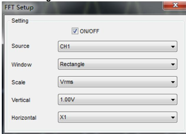
You can select the Source channel, Window type, FFT vertical scale units, vertical scale and FFT Zoom factor. It displays only one FFT spectrum at a time.
