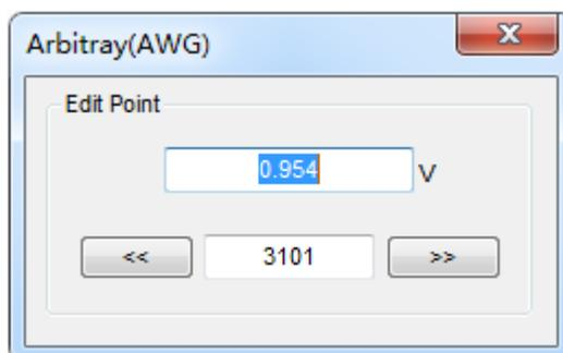
After the completion of the set, click "Download" to output Arbitrary Waveform.
