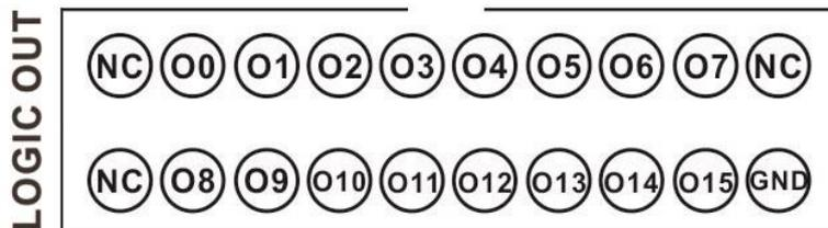
The user can edit the 00-15 high-low level, and output by LOGIC OUT port.
