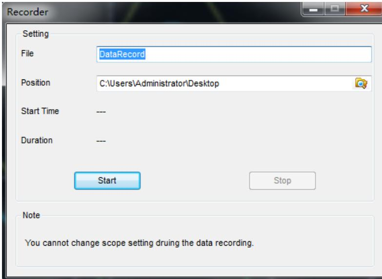
This function can record input waveform from CH1, CH2, CH3 and CH4.
