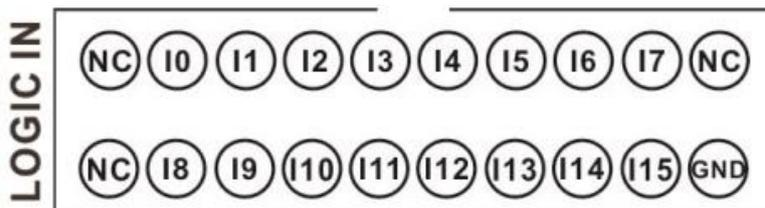
DSO3000A (DSO3104A, DSO3204A, DSO3254A) has 16 signals, I0-I15, Corresponding to the software on the display is D0 - D15.
