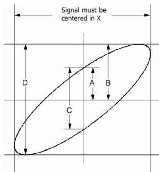
$\sin\theta = A/B$  or  $C/D$ , where  $\theta$  = phase shift (in degrees) between the two signals.
