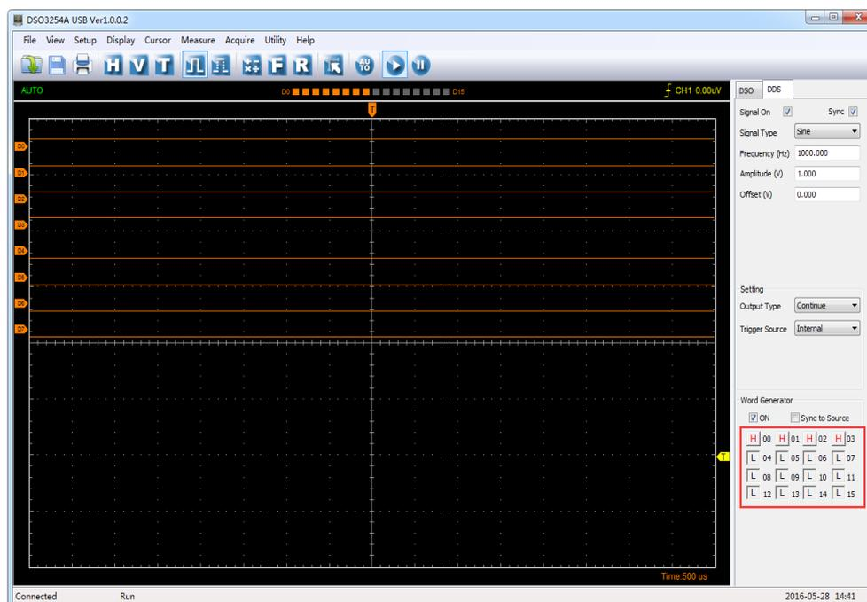
For example, set high eight to HHHLLLLL to LOGIC analyzer LOGIC IN port. The measurement result as following figure.
