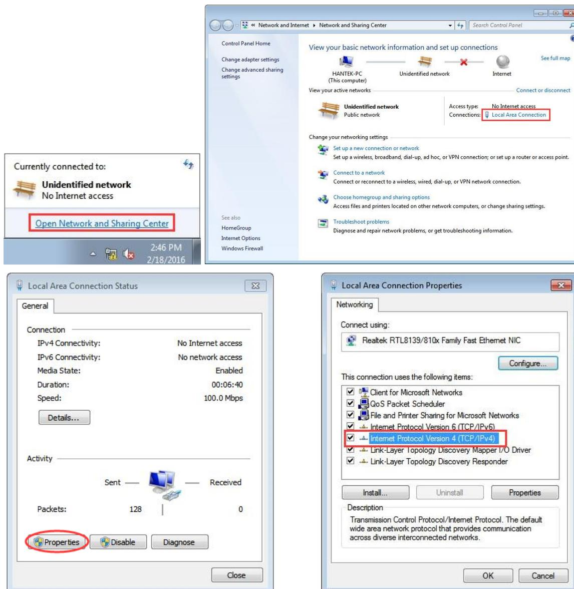
3) Set PC's IP to 192.168.1.2 or others (192.168.1.2~192.168.1.255) except 192.168.1.127. For example, the IP of the device is 192.168.1.32. Set Subnet mask in default.
