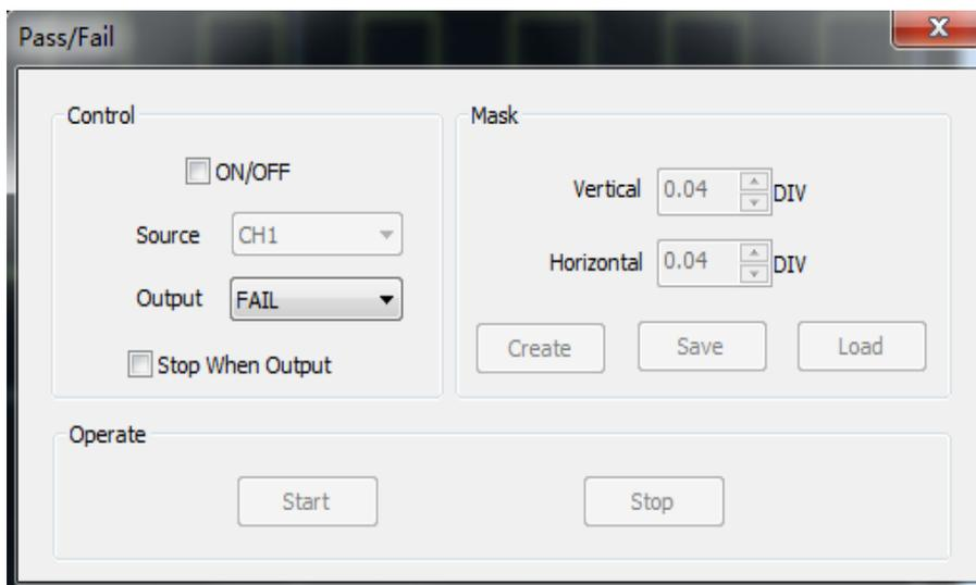
The **Pass/Fail** function monitors changes of signals and outputs pass or fail signals by comparing the input signal with the pre-created mask.
