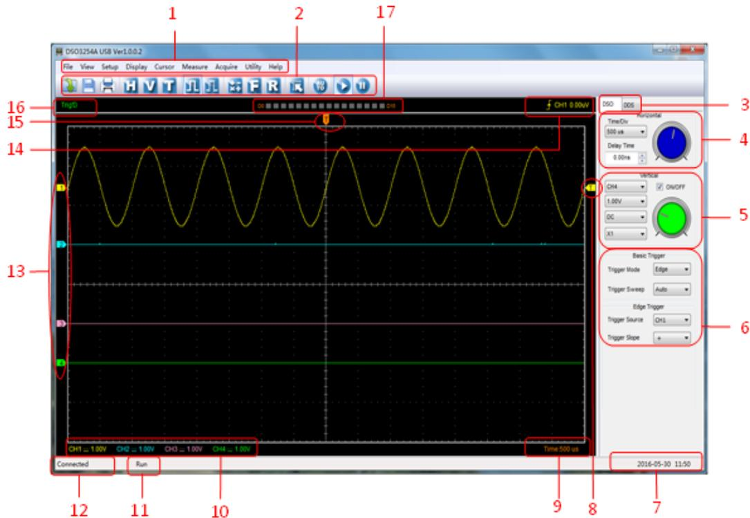
In addition to displaying waveforms, the display area is filled with many details about the waveform and the oscilloscope control settings.
