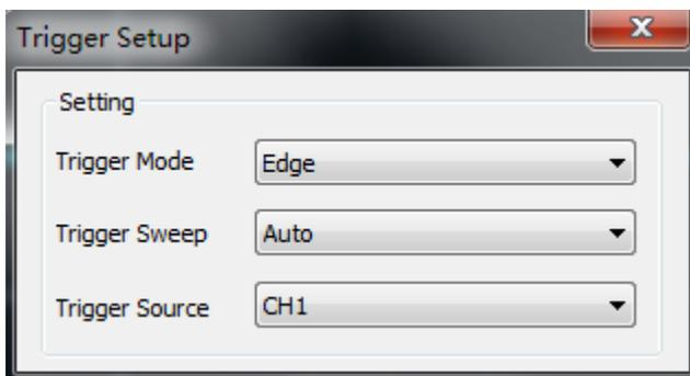
The user can also change the trigger setting on trigger panel in sidebar.
