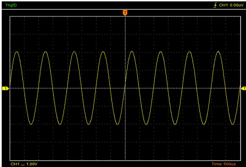
If the **Dots** type mode is selected, the waveform will be displayed as following figure.
