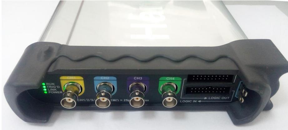
**CH1/CH2/CH3/CH4:** Input connectors for waveform display.
