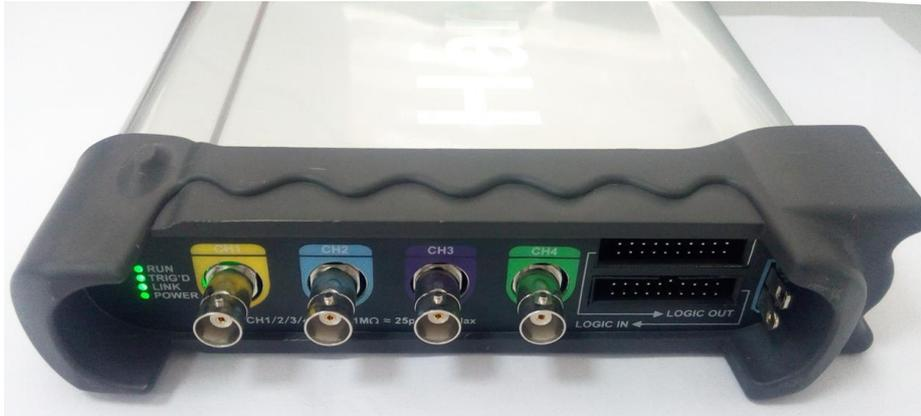
**CH1/CH2/CH3/CH4:** Input connectors for waveform display.
