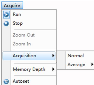
**Normal:** In this acquisition mode, the oscilloscope samples the signal in evenly spaced intervals to construct the waveform.
