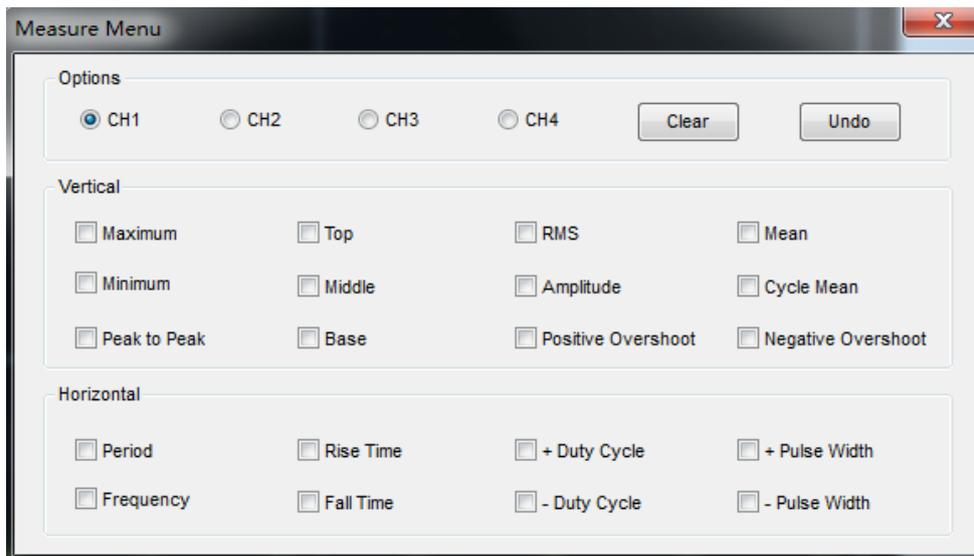
The oscilloscope provides 20 parametric auto measurements (12 voltage and 8 time measurements).
